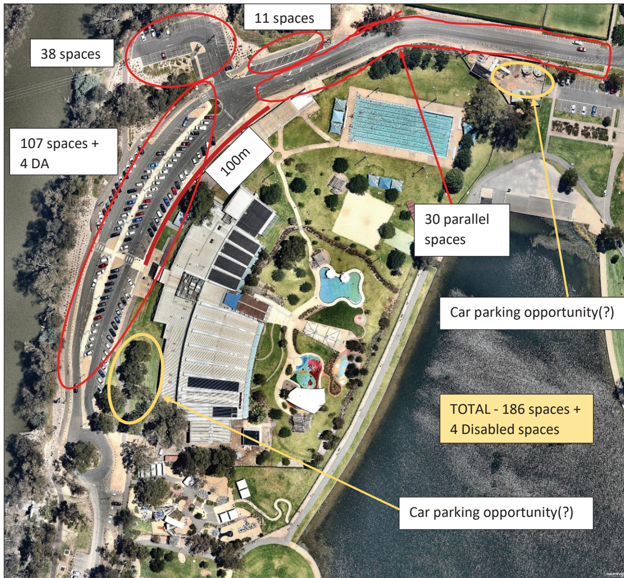
Figure 19: Aquamoves Aerial Photo of Existing Shared Area Car Parks
