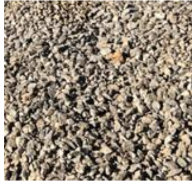
Image 13: Rock that is 20 – 40mm in size and free from dust and fines is used to backfill trenches
